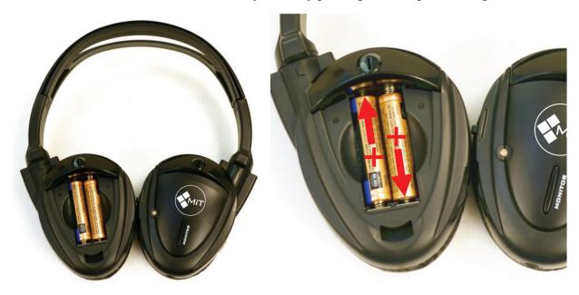
Install AAA batteries with the + (positive) end as indicated above. Re-install battery cover.
